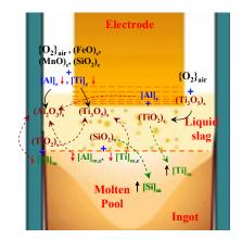
**Fig.2.** Schematic of the Al, Ti, burning loss and Si enrichment behavior during ESR process.
