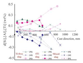
**Fig.3.** Effect of slag on[Al], [Ti] losses using: Ti-free slag 4Ti slag and mixed slag.
