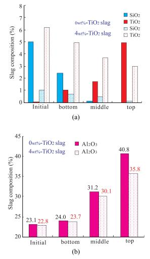
**Fig.5.** Variations of (a)  $SiO_2$ ,  $TiO_2$  and (b)  $Al_2O_3$  in slag for different slags.
